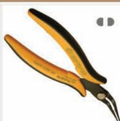
**PN2002 PM:** Smooth, 45° angled long nose pliers with rounded external edges. Thanks to its shape, it gives a wide angle of vision of the work area. Steel thickness 2.0mm. ESD-safe handles version available .
