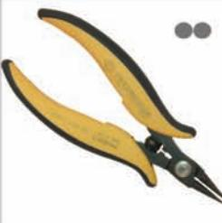
**PN 5025/3:** Smooth rounded short nose pliers, ideal for the handling of components in high density areas without causing damage. Tips diameter 1.0 mm. Nose length 20mm. Steel thickness 5.0mm. ESD-safe handles version available.
