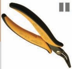
**PNB 2008:** Smooth flat long nose pliers bent at 45°. Thanks to its shape, it gives a wide angle of vision of the work area and suitable for the handling of components in difficult to reach areas. Steel thickness 3.0mm. ESD-safe handles version available.
