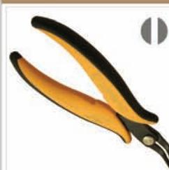
**PNB 2017:** Serrated flat, externally rounded nose pliers bent at 45°, suitable for the handling of components in difficult to reach areas. Steel thickness 3.0mm. ESD-safe handles version available.
