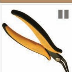
**PNB 2007:** Serrated flat long nose pliers bent at 45°. Thanks to its shape, it gives a wide angle of vision of the work area and suitable for the handling of components in difficult to reach areas. Steel thickness 3.0mm. ESD-safe handles version available.
