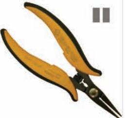
**PN 5008:** Smooth, flat, long nose pliers, ideal for the handling of components in poorly accessible areas and where a strong grip is needed. Steel thickness 5.0mm.
