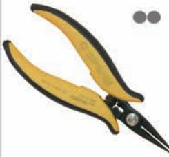
**PN 5025/2:** Smooth rounded long nose pliers, ideal for the handling of components in high density areas without causing damage. Tips diameter 1.0 mm. Nose length 26mm. Steel thickness 5.0mm. ESD-safe handles version available.
