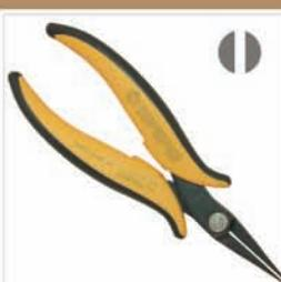
**PN 2017:** Serrated flat, long nose pliers, with rounded external edges suitable for the handling of components in high density areas without causing damage. Steel thickness 3.0mm. ESD-safe handles version available.
