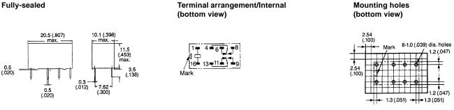
Note: 1. Z and [\_\_] indicate mounting orientation marks. 2. A tolerance of  $\pm 0.10$  (0.004) applies to the above dimensions.
