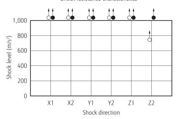
Shock application time: 6±1ms, half-sine wave Test condition: Coil energized and de-energized
