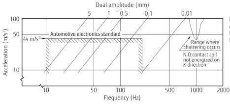
Frequency: 10 to 2000Hz Acceleration: 100m/s² max.
