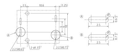
Tolerance of PC board mounting hole layout: ±0.1 unless otherwise specified.
