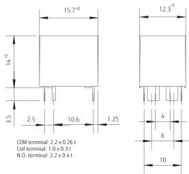
Dimensions of the terminals do not include thickness of pre-solder.
