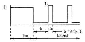
3rd wire signal Run : Square Wave Locked : Vm
