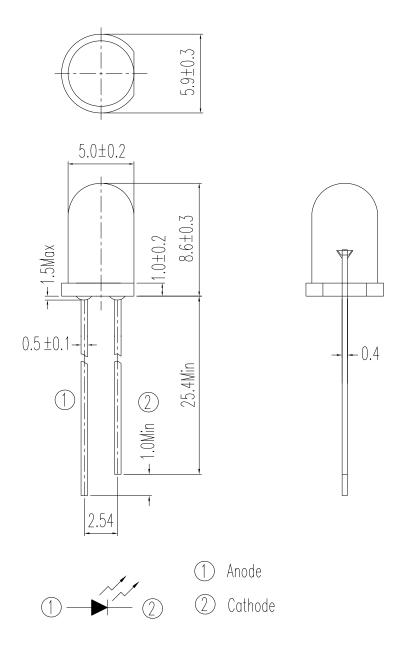
Note: Tolerances unless dimensions ±0.25mm
