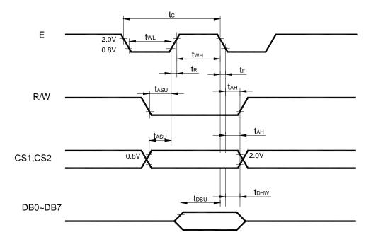
Figure 5.0 MPU write timing
