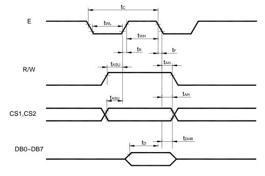
Figure 6.0 MPU Read timing
