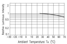
Fig.5 Luminous Intensity vs.
