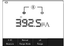
Picture 5-10 Measurement of AC Current lower than 4mA
