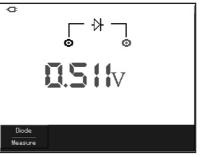
Picture 5-2 Diode Measurement
