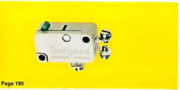
V3F – silver contacts and V3FN – platinum contacts. Maximum continuous working temperature 240°C. Electrical Ratings table 2 below
