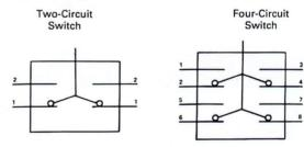
Both diagrams indicate the 'at rest' position of the switch.
