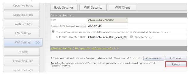
Remark 3: After VONETS device sets the WAN port to access the WiFi hotspot in the routing mode, its LAN port IP is still 192.168.254.254, and the terminal device also obtains the IP address of the same network segment, can login configuration page by 192.168.254.254 or http://vonets.cfg.
