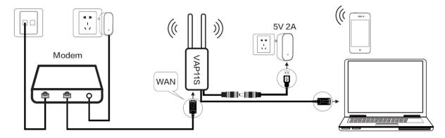
VONETS device is used as WiFi router, WAN port can be set to connect to the WiFi
