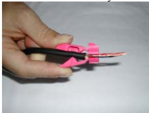
Step 4. Fit the cable into the "Jaws" cable clamp.
