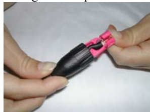
Step 8. Push boot on to "Jaws" clamp to hold conductors in place.
