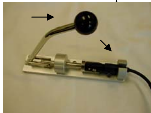
Step 11. Terminate by screwing on the boot or popping on with the Amphenol Tool.
