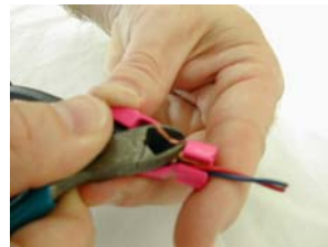
Step 6. Trim shield wire to ensure no contact is made with shell.
