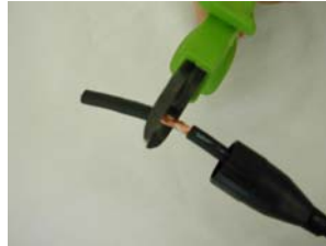
Step 2. Strip cable outer jacket Approx 1.25" (30-35mm)
