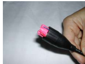
Step 9. Boot holding conductors in place.
