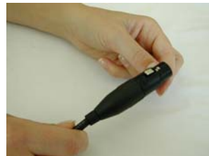
Step 12. Terminated IDC connector.
