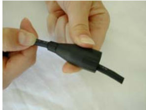
Step 1. Push cable through boot assembly.
