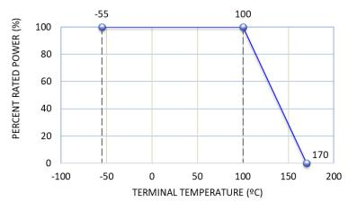
Operating temperature range of -55 $^{\circ}$ C to 170 $^{\circ}$ C. Storage condition: 5 $^{\circ}$ C ~ 35 $^{\circ}$ C, humidity of 40% ~ 75%.
