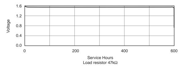
Average Service Capacity: 20 mAh (rated capacity at  $47k\Omega$  load, cut off voltage 1.3V at  $24^{\circ}C$ )
