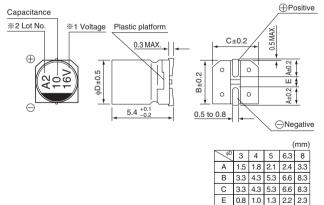
%1. Voltage mark for 6.3V is [6V]. In case of marking for φ3 units, "V" for rated voltage is omitted.
