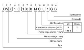
• In the case of size  $\phi$ 3 in ( ),parentheses, use WX in the 2nd and 3rd 2 digit and put a in the 12th digit of type numbering system.
