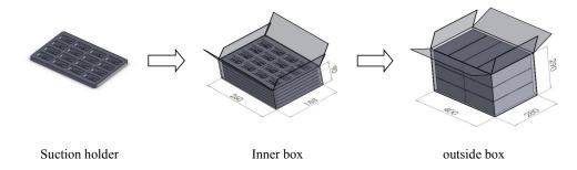
Packaging of Snap-in and Lead Types Supercapacitor:
