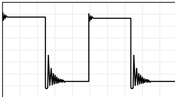
(b) C_L = 260 \text{ pF} , R_L = \text{NO LOAD}
