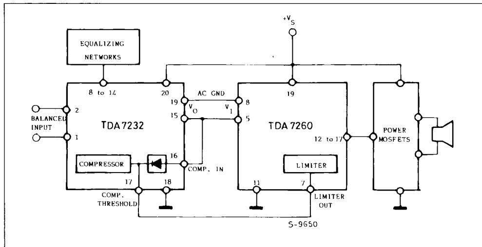
Figure 16 : 25 W Application Circuit.
