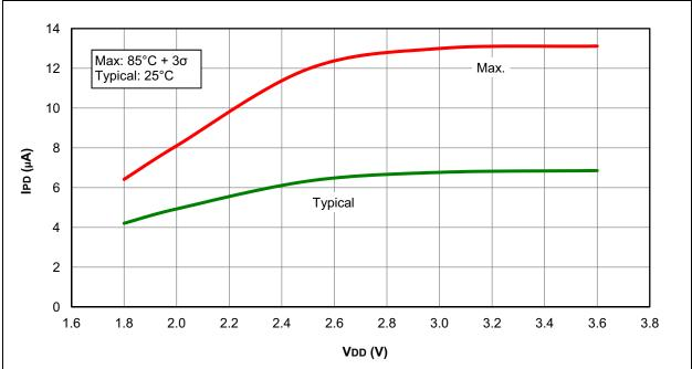
FIGURE 31-42: IPD, CAPACITIVE SENSING (CPS) MODULE, MEDIUM-CURRENT RANGE, CPSRM = 0, CPSRNG = 10, PIC16F1933 ONLY
