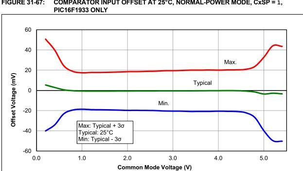
COMPARATOR INPUT OFFSET AT 25°C, NORMAL-POWER MODE, CxSP = 1, FIGURE 31-67:
