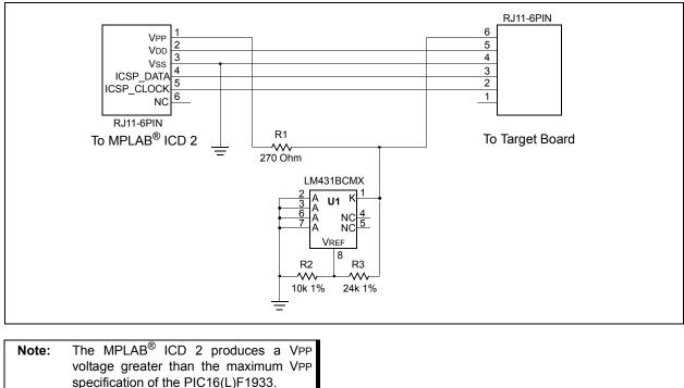
FIGURE 28-1: VPP LIMITER EXAMPLE CIRCUIT
