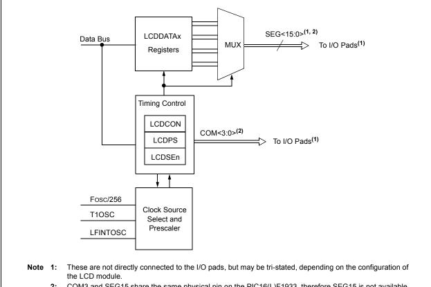
COM3 and SEG15 share the same physical pin on the PIC16(L)F1933, therefore SEG15 is not available 2: when using 1/4 multiplex displays.
