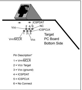
Another connector often found in use with the PICkit<sup>™</sup> programmers is a standard 6-pin header with 0.1 inch spacing. Refer to Figure 28-3.
