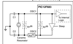
Note 1: A series resistor (Rs) may be required for ceramic resonators with low drive level.
