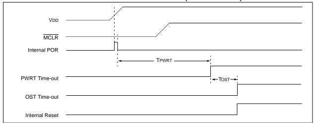
FIGURE 12-5: TIME-OUT SEQUENCE ON POWER-UP (DELAYED MCLR)
