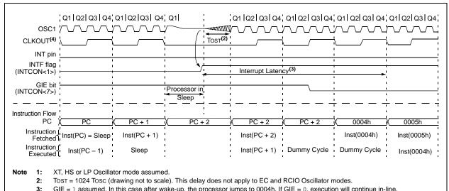
CLKOUT is not available in XT, HS, LP or EC Oscillator modes, but shown here for timing reference.
