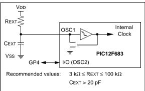
The RC oscillator frequency is a function of the supply voltage, the resistor (REXT) and capacitor (CEXT) values and the operating temperature. Other factors affecting the oscillator frequency are:
