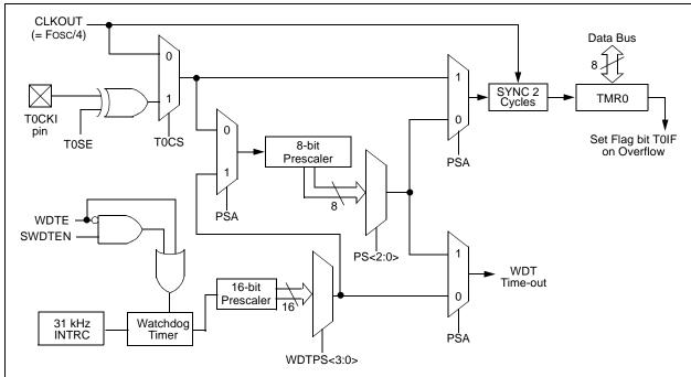
Note 1: T0SE, T0CS, PSA and PS<2:0> are bits in the Option register, WDTPS<3:0> are bits in the WDTCON register.
