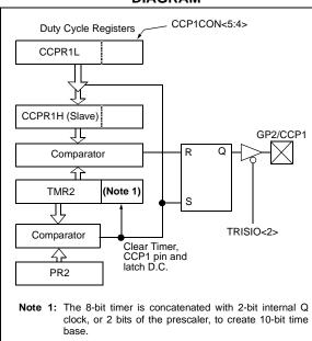
A PWM output (Figure 11-4) has a time base (period) and a time that the output stays high (duty cycle). The frequency of the PWM is the inverse of the period (1/period).
