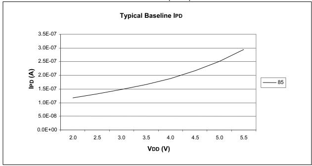
**FIGURE 13-3:** TYPICAL IPD vs. VDD OVER TEMP (+125°C)
