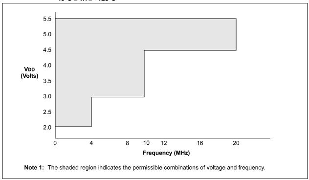
FIGURE 12-2: PIC12F675 WITH A/D ENABLED VOLTAGE-FREQUENCY GRAPH,  $-40^{\circ}\text{C} \le \text{Ta} \le +125^{\circ}\text{C}$
