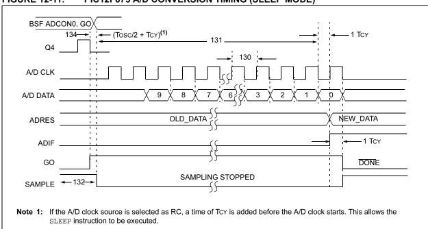
FIGURE 12-11: PIC12F675 A/D CONVERSION TIMING (SLEEP MODE)
