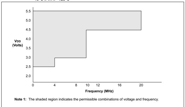
FIGURE 12-3: PIC12F675 WITH A/D ENABLED VOLTAGE-FREQUENCY GRAPH,  $0^{\circ}C \le TA \le +125^{\circ}C$
