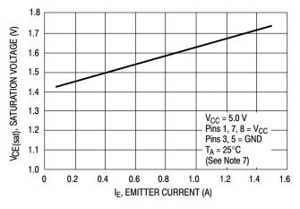
Figure 5. Emitter Follower Configuration Output **Saturation Voltage versus Emitter Current**
