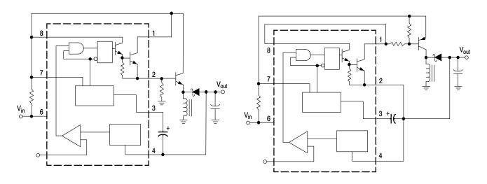
Figure 14. External Current Boost Connections for I<sub>C</sub> Peak Greater than 1.5 A
