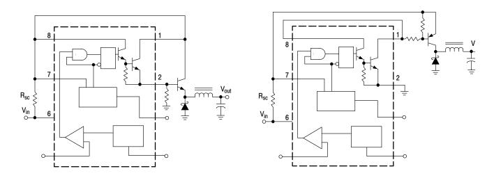
Figure 12. External Current Boost Connections for  $I_{\mbox{\scriptsize C}}$  Peak Greater than 1.5 A
