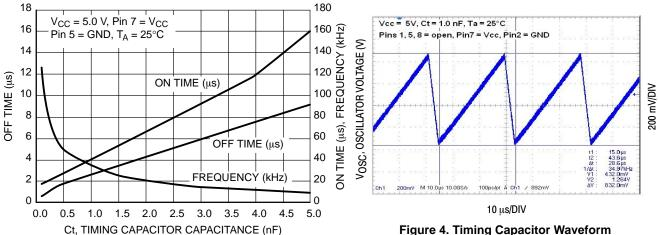
Figure 3. Oscillator Frequency
