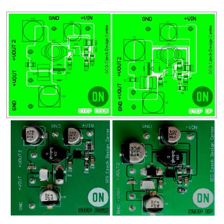
Figure 16. Printed Circuit Board for DFN Device
