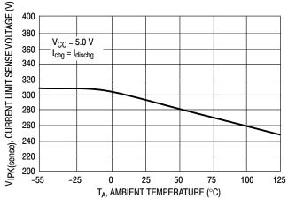
Figure 7. Current Limit Sense Voltage versus Temperature
