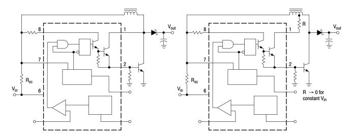
Figure 10. External Current Boost Connections for I<sub>C</sub> Peak Greater than 1.5 A
