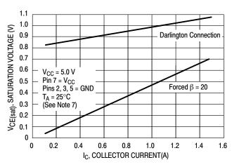
**Figure 6. Common Emitter Configuration Output Switch Saturation Voltage versus Collector Current**
