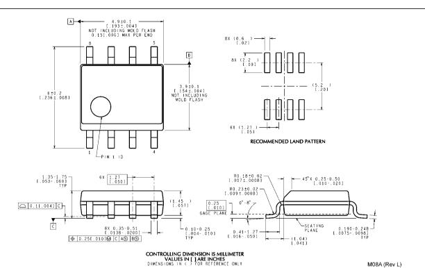
Small Outline (SO-8) Package Order Number LM285M-1.2, LM285BXM-1.2, LM285BYM-1.2 LM385M-1.2, LM385BM-1.2, LM385BXM-1.2, LM385BYM-1.2 NS Package Number M08A
