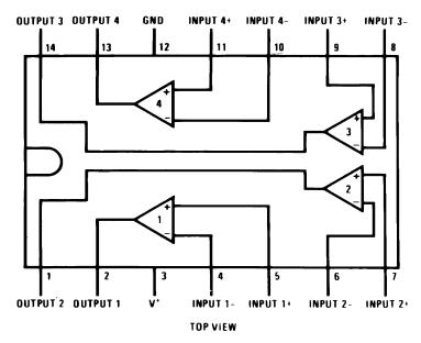
Dual-In-Line Package - SOIC/PDIP See Package Number D and NFF
