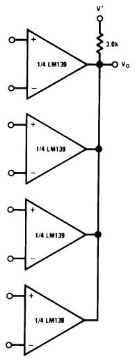
Figure 16. ORing the Outputs
