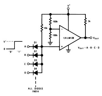
Figure 15. Large Fan-In AND Gate
