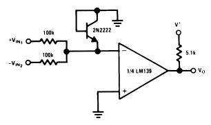
Figure 23. Comparing Input Voltages of Opposite Polarity
