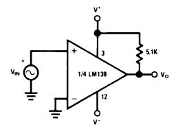
Figure 30. Zero Crossing Detector
