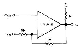
Figure 18. Non-Inverting Comparator with Hysteresis
