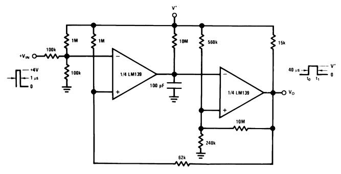
Figure 13. One-Shot Multivibrator with Input Lock Out
