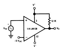
Figure 31. Comparator With a Negative Reference
