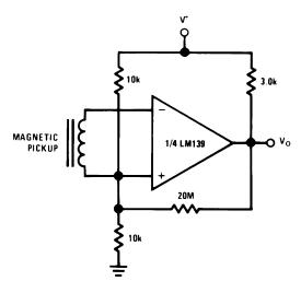
Figure 27. Transducer Amplifier
