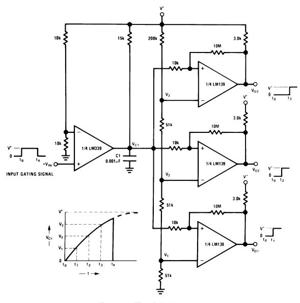
Figure 17. Time Delay Generator
