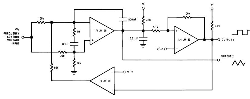
$V^{+} = +30 \text{ V}_{DC}$ 250 mV<sub>DC</sub>  $\leq$  V<sub>C</sub>  $\leq$  +50 V<sub>DC</sub> 700 Hz  $\leq$  f<sub>O</sub>  $\leq$  100 kHz
