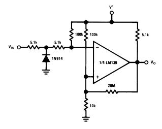
Figure 28. Zero Crossing Detector (Single Power Supply)
