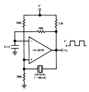
Figure 25. Crystal Controlled Oscillator
