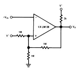
Figure 19. Inverting Comparator with Hysteresis
