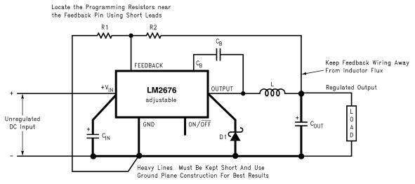
Figure 22. Basic Circuit for Adjustable Output Voltage Applications
