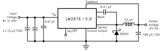
Figure 16. Basic Circuit for All Output Voltage Versions
