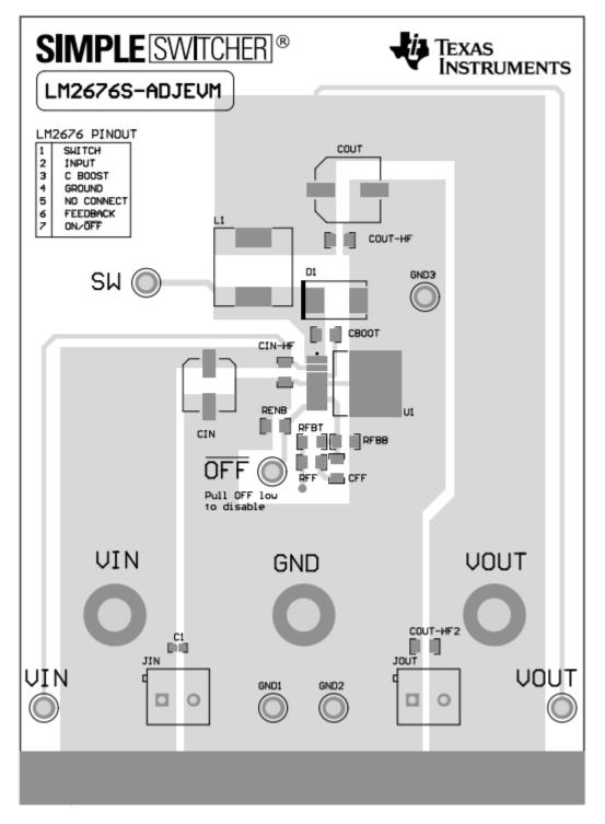
Figure 24. LM2676 Layout Example
