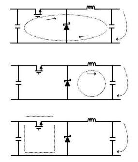
Figure 23. Typical Current Flow on a Buck Converter
