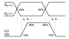
Figure 2. Switching Time Waveform Definitions
