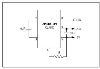
Figure 8. Splitting +15V with an ICL7660, 95% Efficiency (Same for -15V)
