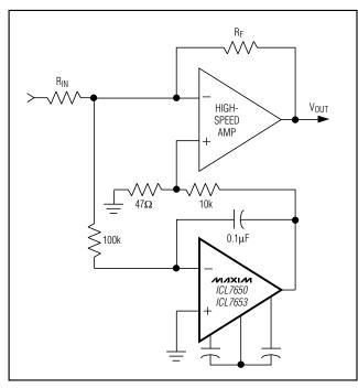
Figure 4. Nulling a High-Speed Amplifier
