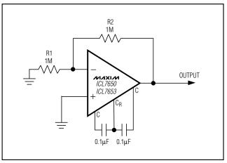
Figure 1. ICL7650 Test Circuit
