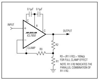
Figure 6. Noninverting Amplifier with Optional Clamp
