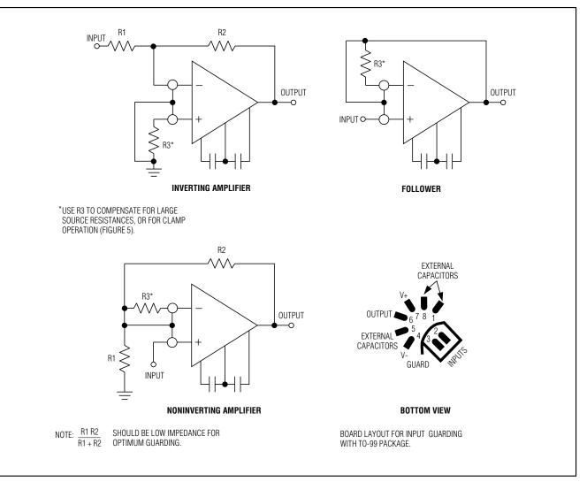
Figure 3. Input Guard Connection
