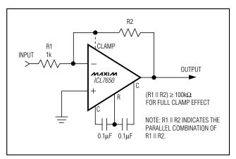
Figure 5. Inverting Amplifier with Optional Clamp
