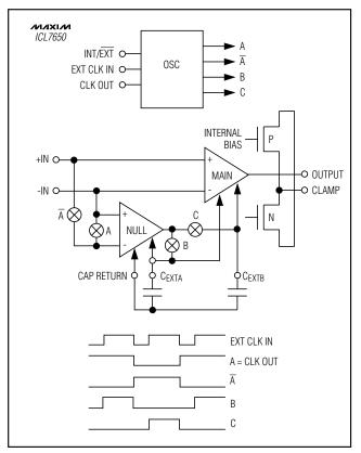
Figure 2. Block Diagram
