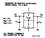
Fig.24 - Capacitance C<sub>IOS</sub> and C<sub>OS</sub>.
