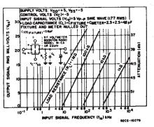
Fig. 8 — Typ. feedthru vs. frequency — switch off.
