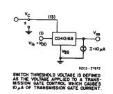
Fig.23 - Switch threshold voltage.
