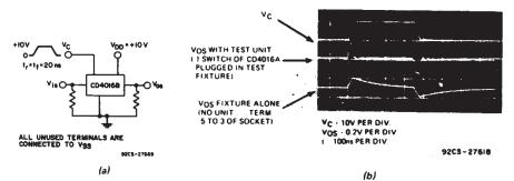
Fig. 20 - Crosstalk-control input to signal output.
