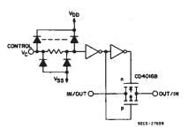
Schematic diagram - 1 of 4 identical sections.
