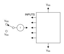
Figure 15. Input Current Test Circuit
