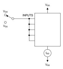
Figure 14. Quiescent Device Current Test Circuit
