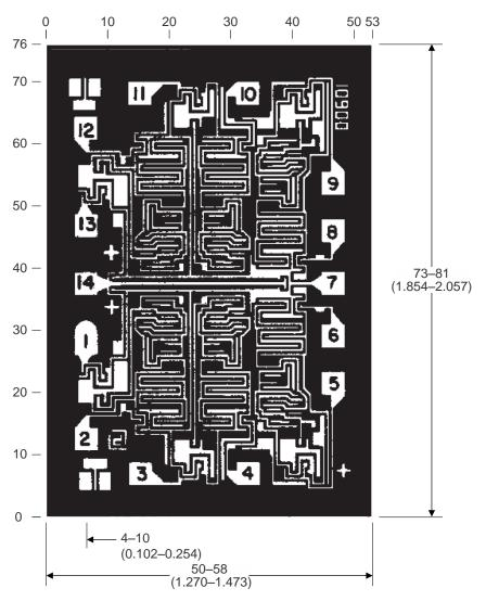
Figure 22. Dimensions and Pad Layout for CD40106BH
