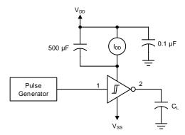
Figure 16. Dynamic Power Dissipation Test Circuit
