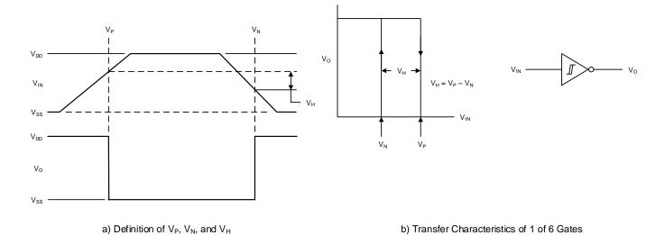
Figure 13. Hysteresis Definition, Characteristics, and Test Set-Up
