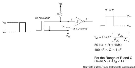
Figure 19. Monostable Multivibrator Schematic and Equations
