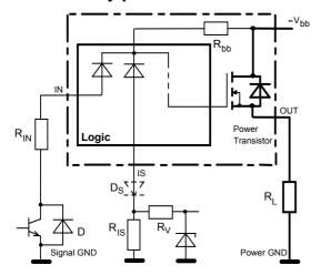
$R_V \ge 1 \text{ k}\Omega$ ,  $R_{IS} = 1 \text{ k}\Omega$  nominal. Add  $R_{IN}$  for reverse battery protection in applications with  $V_{bb}$  above
