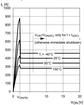
In case of  $V_{ON} > V_{ON(SC)}$  (typ. 6 V) the device will be switched off by internal short circuit detection.
