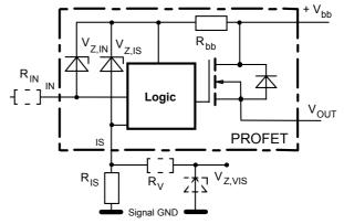
$R_{bb}$  = 120  $\Omega$  typ.,  $V_{Z,IN}$  =  $V_{Z,IS}$  = 66 V typ.,  $R_{IS}$  = 1 k $\Omega$  nominal. Note that when overvoltage exceeds 71 V typ. a voltage above 5V can occur between IS and GND, if  $R_V$ ,  $V_{Z,VIS}$  are not used.
