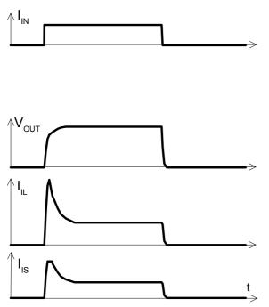
Sense current saturation can occur at very high inrush currents (see  $I_{\text{IS,lim}}$  on page 6).
