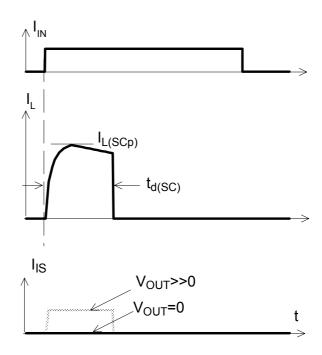
Shut down remains latched until next reset via input.
