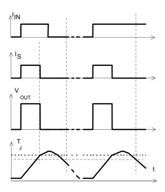
**Figure 5:** Undervoltage restart of charge pump, overvoltage clamp
