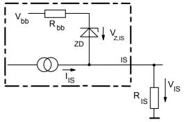
$V_{\rm Z,IS}$  = 66 V (typ.),  $R_{\rm IS}$  = 1 k $\Omega$  nominal (or 1 k $\Omega$  /n, if n devices are connected in parallel).  $I_{\rm S}$  =  $I_{\rm L}/k_{\rm ilis}$  can be only driven by the internal circuit as long as  $V_{\rm out}$  -  $V_{\rm IS}$  > 5V. If you want to measure load currents up to  $I_{\rm L(M)}$ ,  $R_{\rm IS}$  should be less than  $\frac{V_{bb}-5V}{I_{L(M)}/K_{ilis}}$ .
