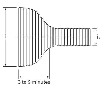
The discharge tube, transformer, choke coil, capacitor, etc., are combined in common discharge lamp circuits. Note that the inrush current may be 20 to 40 times, especially if the power supply impedance is low in the high power factor type.
