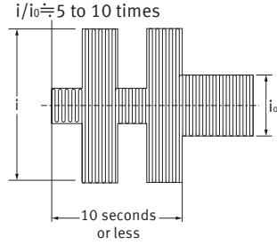
(4) Motor Load  $i/i_0 = 5$  to 10 times
