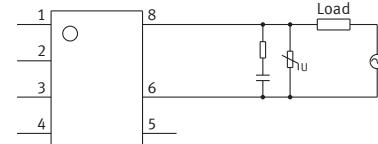
Note: Connection of an external resistor, etc., to terminal No. 5 (gate) is not necessary.
