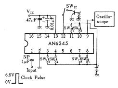
• PG Output(H),(L): Apply clock pulses to the Pin① in accordance with the Divide Select List and measure Pin③ output per item.
