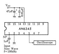
• Input signal when Pin 5 output is normally made.
