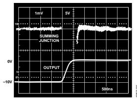
Figure 30. Settling Characteristics for AD712 with AD565A, Full-Scale Positive Transition
