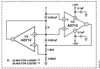
Figure 51. FDNR for 9-Pole Chebychev Filter
