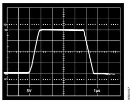
Figure 27. Unity-Gain Inverter Pulse Response (Large Signal)
