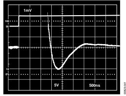
Figure 41. Positive Settling Characteristics for AD712 with AD7545
