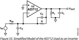
In either case, Capacitance Cx causes the system to go from a one-pole to a two-pole response; this additional pole increases settling time by introducing peaking or ringing in the op amp output. Because the value of C<sub>x</sub> can be estimated with reasonable accuracy, Equation 2 can be used to choose a small capacitor (C<sub>F</sub>) to cancel the input pole and optimize amplifier response. Figure 34 is a graphical solution of Equation 2 for the AD712 with  $R = 4 k\Omega$ .
