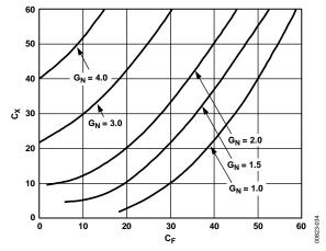
Figure 34. Value of Capacitor C<sub>F</sub> vs. Value of C<sub>X</sub>
