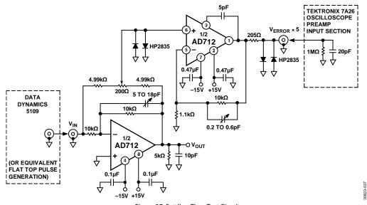
Figure 37. Settling Time Test Circuit
