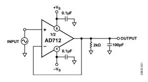
Figure 21. THD Test Circuit
