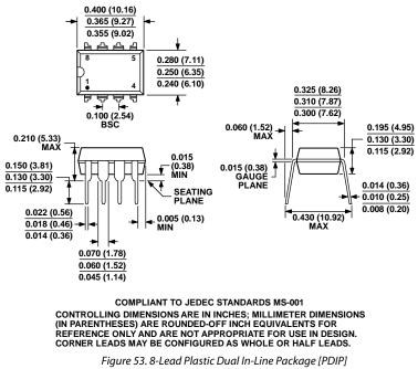
(N-8) Dimensions shown in inches and (millimeters)
