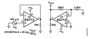
Figure 22. Crosstalk Test Circuit
