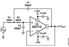
Figure 48. Second-Order Low-Pass Filter
