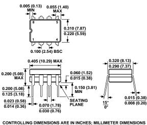
CONTROLLING DIMENSIONS ARE IN INCHES; MILLIMETER DIMENSIONS (IN PARENTHESES) ARE ROUNDED-OFF INCH EQUIVALENTS FOR REFERENCE ONLY AND ARE NOT APPROPRIATE FOR USE IN DESIGN.
