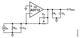
Figure 32. Simplified Model of the AD712 Used as a Current-Out DAC Buffer
