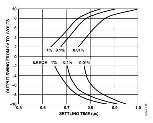
Figure 16. Output Swing and Error vs. Settling Time
