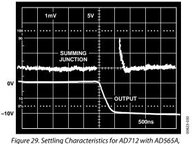
gure 29. Settling Characteristics for AD712 with AD565A Full-Scale Negative Transition
