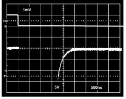
Figure 42. Negative Settling Characteristics for AD712 with AD7545
