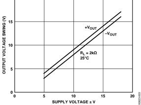
Figure 3. Output Voltage Swing vs. Supply Voltage
