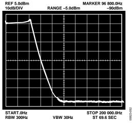
Figure 52. High Frequency Response for 9-Pole Chebychev Filter
