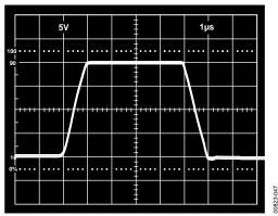
Figure 47. Transient Response  $R_L = 2 k\Omega$ ,  $C_L = 500 pF$
