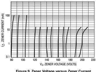
Figure 9. Zener Voltage versus Zener Current V<sub>Z</sub> = 82 thru 200 Volts
