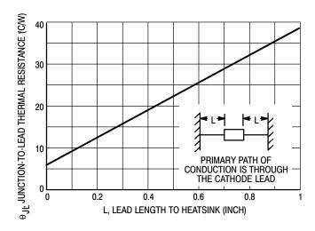
Figure 1. Typical Thermal Resistance
