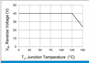
**Fig.5 Operating Temperature Derating**
