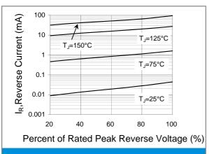
Fig.3 Typical Reverse Characteristics
