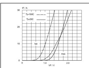
Fig.5. BY359-1500 forward characteristic  $I_F = f(V_F)$ ; parameter  $T_j$
