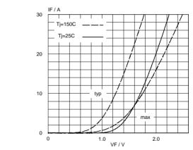
Fig.6. BY359-1500S forward characteristic  $I_F = f(V_F)$ ; parameter  $T_j$
