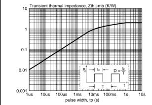
Fig.4. Transient thermal impedance  $Z_{th} = f(t_p)$
