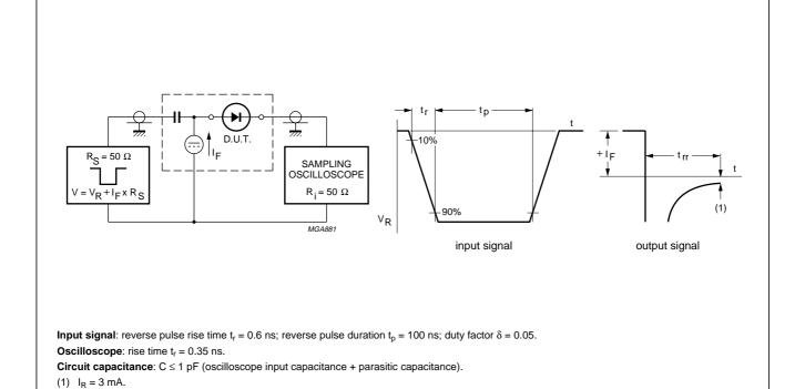
Fig.10 Reverse recovery voltage test circuit and waveforms.
