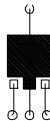
b. 95^\circ\text{C/W} when mounted on a 0.066\text{ in}^2 pad of 2oz Cu.
