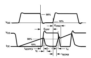
FIGURE 25. SWITCHING TEST WAVEFORMS
