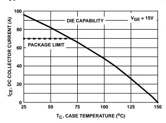
FIGURE 1. DC COLLECTOR CURRENT vs CASE TEMPERATURE
