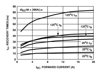
FIGURE 20. RECOVERY TIMES vs FORWARD CURRENT
