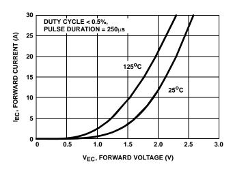
FIGURE 19. DIODE FORWARD CURRENT vs FORWARD VOLTAGE DROP
