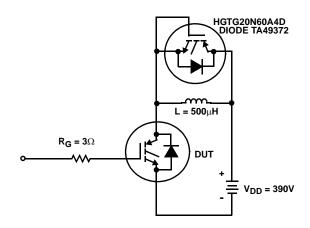
FIGURE 24. INDUCTIVE SWITCHING TEST CIRCUIT
