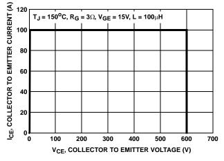
FIGURE 2. MINIMUM SWITCHING SAFE OPERATING AREA
