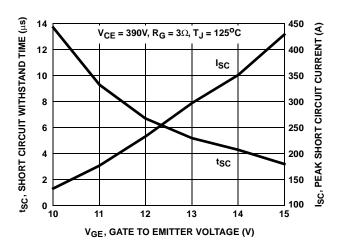
FIGURE 4. SHORT CIRCUIT WITHSTAND TIME
