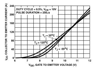
FIGURE 13. TRANSFER CHARACTERISTIC
