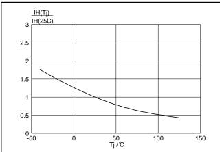
Fig.9. Normalised holding current  $I_H(T_i)/I_H(25\,^{\circ}C)$ , versus junction temperature  $T_j$ .
