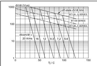
Fig.12. Typical commutation dV/dt versus junction temperature, parameter commutation  $dI_{\tau}/dt$ . The triac should commutate when the dV/dt is below the value on the appropriate curve for pre-commutation  $dI_{\tau}/dt$ .
