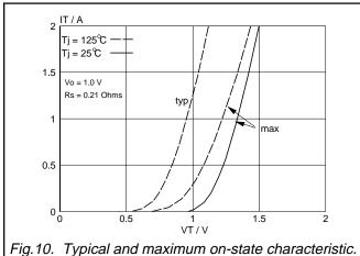
Fig.10. Typical and maximum on-state characteristic.
