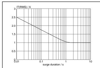
Fig.5. Maximum permissible repetitive rms on-state current  $I_{T(RMS)}$ , versus surge duration, for sinusoidal currents, f = 50 Hz;  $T_{lead} \le 51$  °C.
