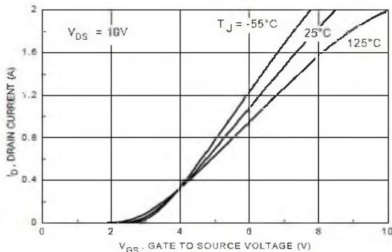
Figure 5. Transfer Characteristics.
