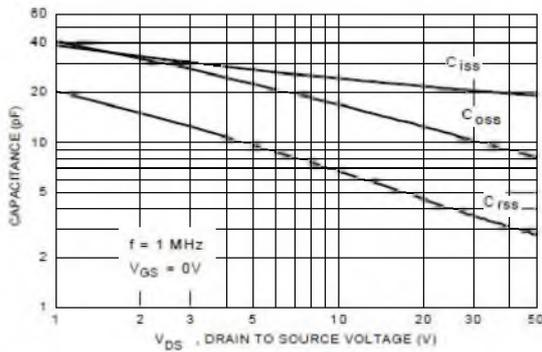
Figure 9. Capacitance Characteristics.
