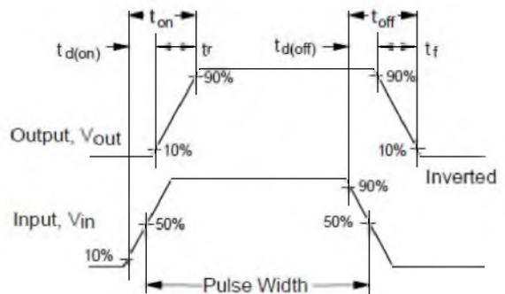
Figure 12. Switching Waveforms.
