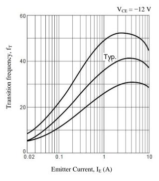
Figure 8. Transition Frequency vs. Emitter Current
