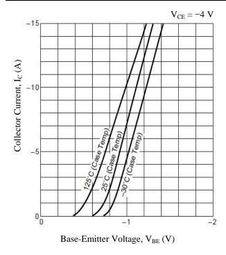
Figure 5. Collector Current vs. Base-Emitter Voltage
