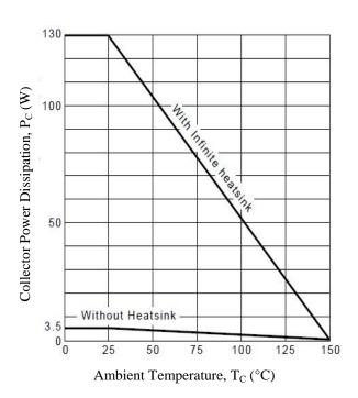
Figure 2. Power Dissipation vs. Ambient Temperature
