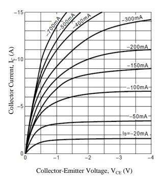
Figure 3. Collector Current vs. Collector-Emitter Voltage
