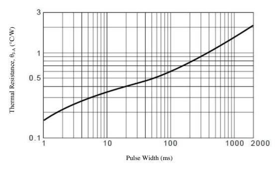
Figure 9. Transient Thermal Resistance
